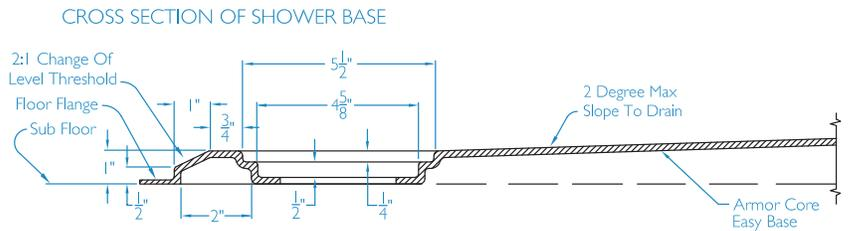
**FEATURES** lbs Dimensional Tolerance ± 3/16". Dimensions needed for site preparation should be measured from the unit. Manufacturer assumes no responsibility for preparatory work.
